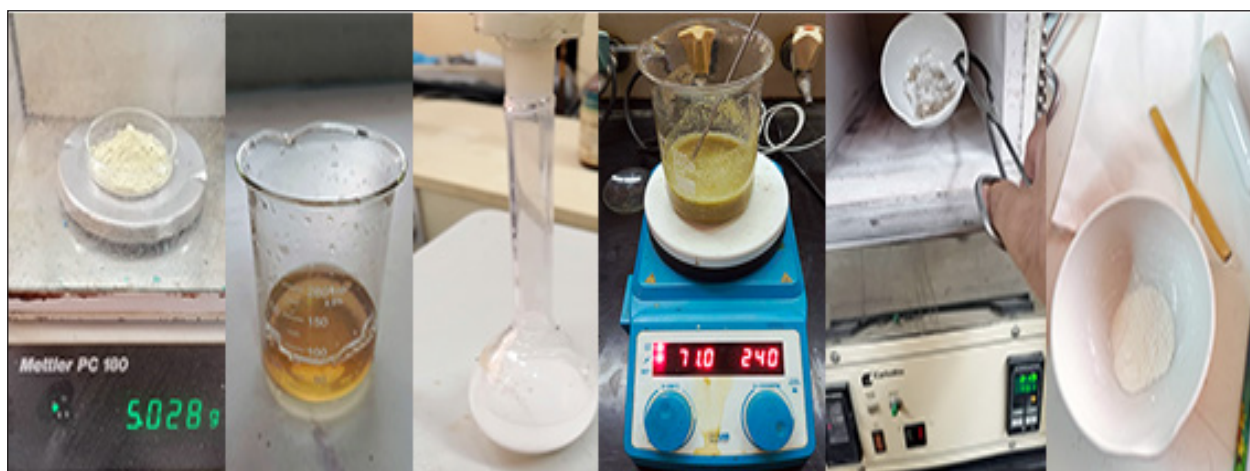
Fig. 1. Sol-Gel method for green synthesis of \text{TiO}_2 NPs
